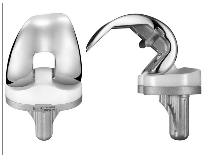
Fig. 1. Femoral component, tibial insert, and tibial component of the LOSPA total knee prosthesis. LOSPA prosthesis requires removal of additional bone from the posterior femoral condyle to add 10 mm posterior condyle at a large posterior radius of the femoral component. In addition, the femoral component has a more rounded contour and a deepened patellar groove to help deep flexion. The posterior surface of the insert is released for deep flexion favoring design.
